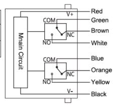
Note: The definition of the output line is based on the actual product label. The image above indicates the status of each wire after power is applied. The default state of Relay 1 will switch before and after power is applied.
